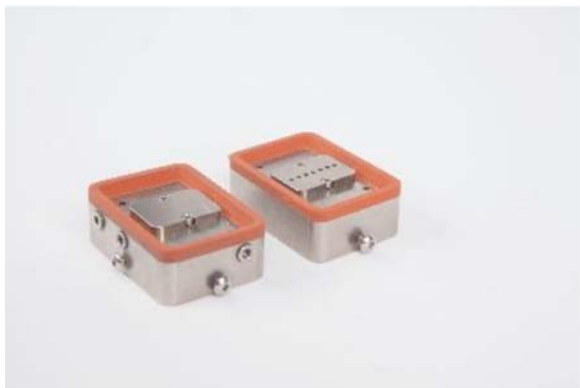
Possible sealing heads to limit the escape of water vapor from test sample overlaps during pressing. Heads are mounted on pressing blocks for the standard apparatus.
