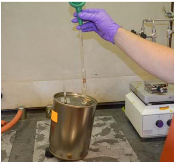
FIG. 2 Draining of Sample Container with No Spout
