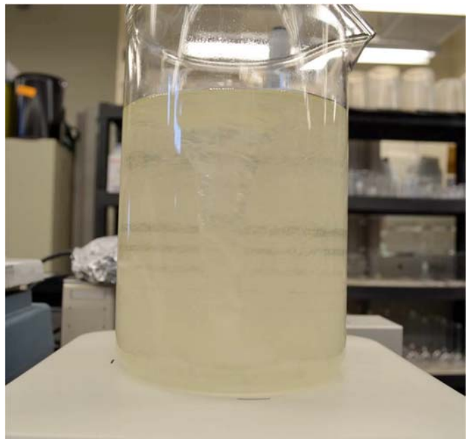
FIG. 4 Inadequate Stir Speed (that is, Bars Still Visible)
