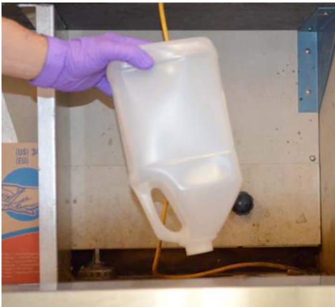
FIG. 1 Draining of Sample Container with a Spout
