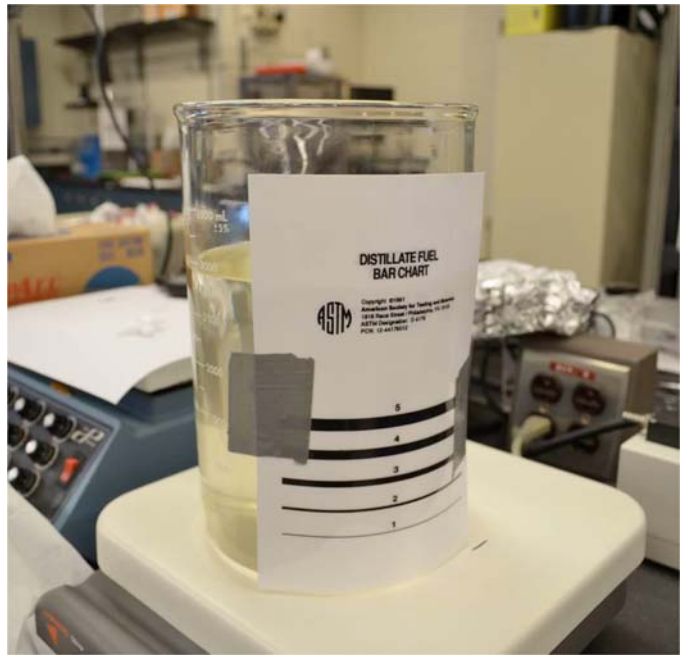
FIG. 3 Taping of Double-Sided Distillate Fuel Bar Chart to 4 L Beaker
