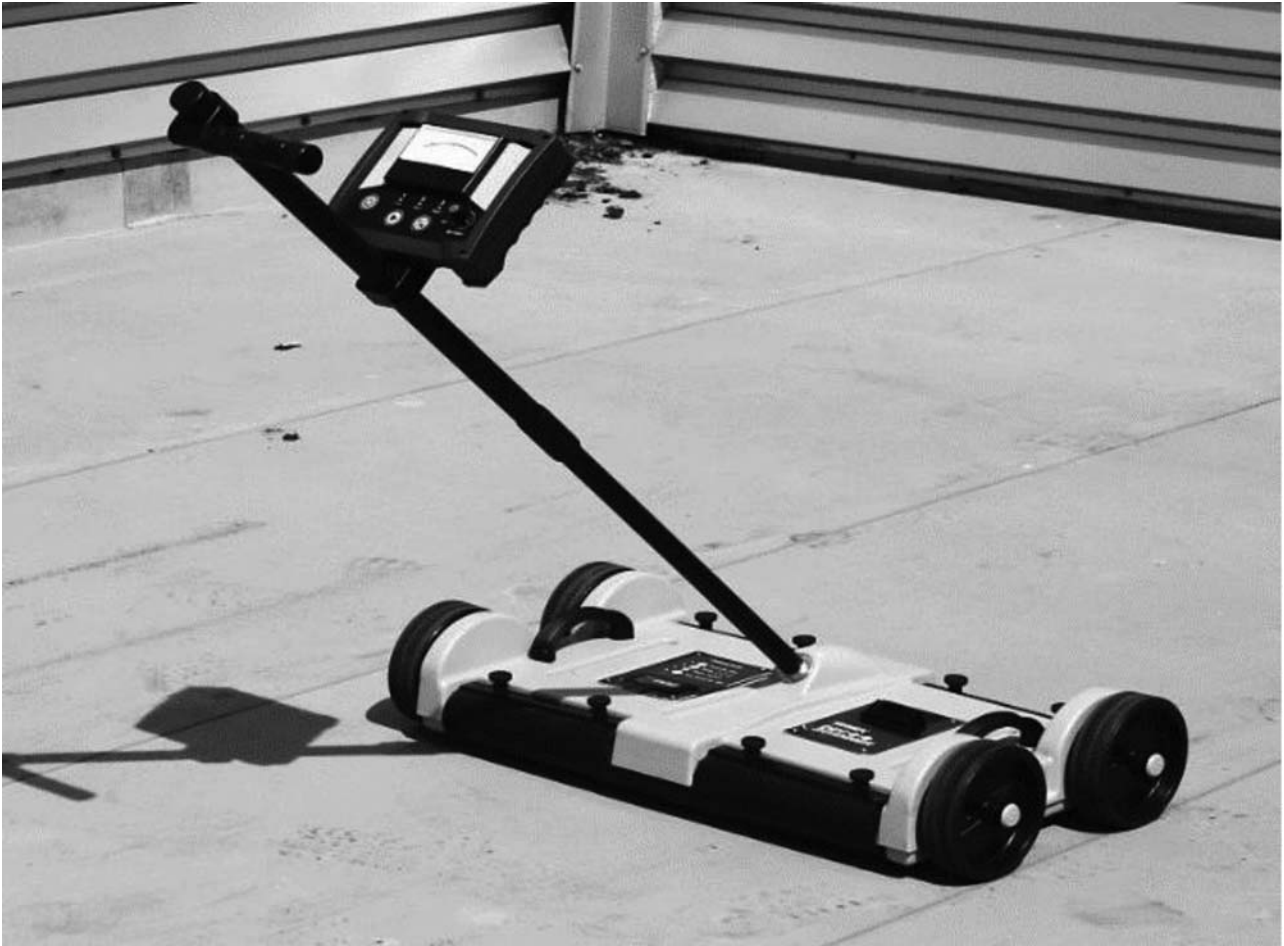
FIG. A1.2 Typical Continuous Impedance Scanner
