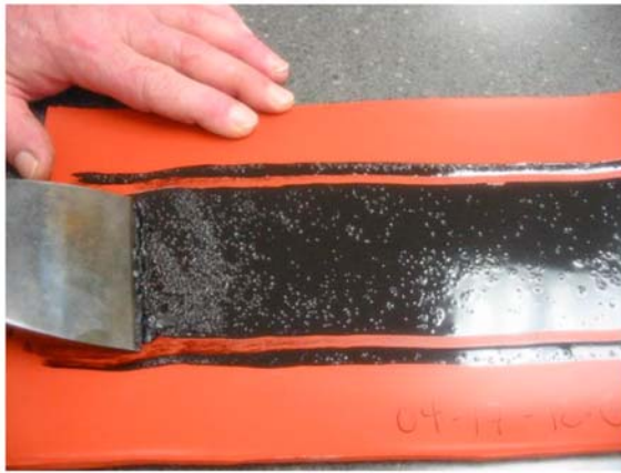
(a) Scraping of emulsified asphalt residue from silicone rubber mat
