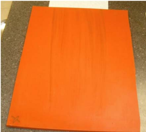
FIG. 4 Example of Silicone Rubber Mat Surface After Wiping Clean, Prior to Re-application of Emulsified Asphalt
