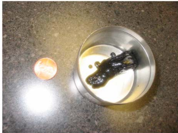
(b) Depositing emulsified asphalt residue in sample tin
