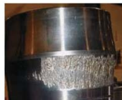
FIG. X2.2 Derivation of Bearing Spall Damage Limit
