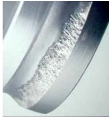
FIG. 2 Typical Bearing Spall
