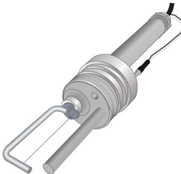
FIG. 3 Close-Up of the Transient Hot Wire Sensor
