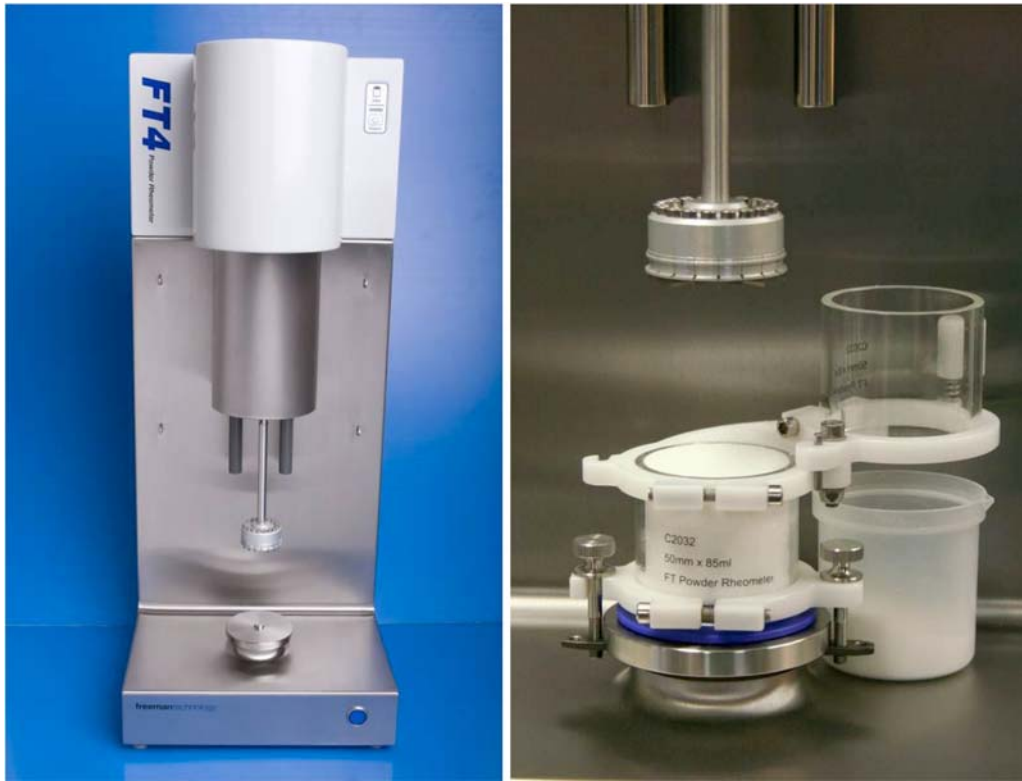
FIG. 1 FT4 Powder Rheometer (The left hand image shows the instrument with the shear head fitted; the right hand image shows the shear head and shear cell vessel.)
