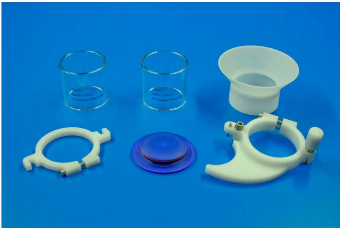
FIG. 4 Components Required to Assemble the 50-mm x 85-mL Shear Cell Vessel
