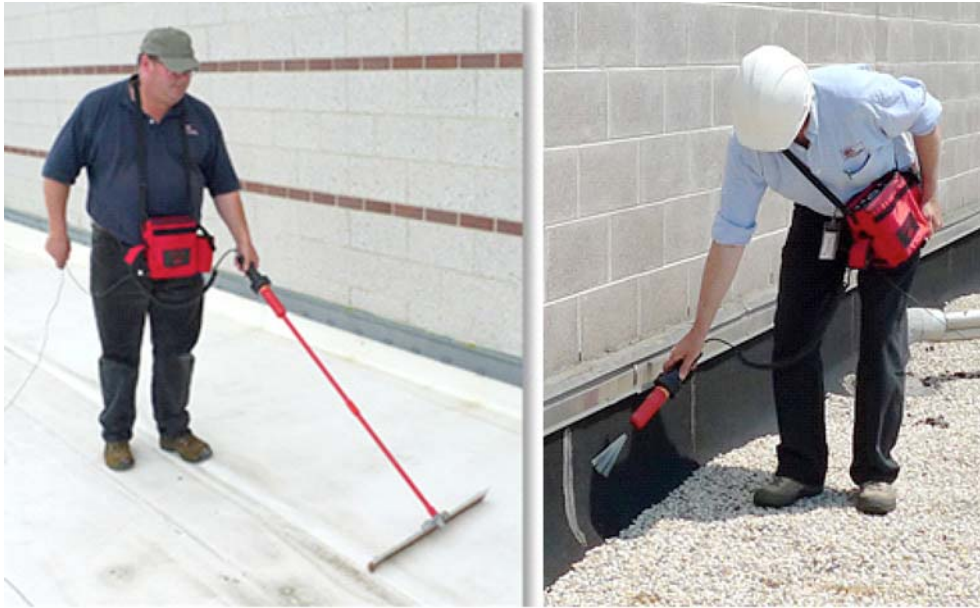
FIG. 7 High Voltage Horizontal and Vertical Membrane Scan
