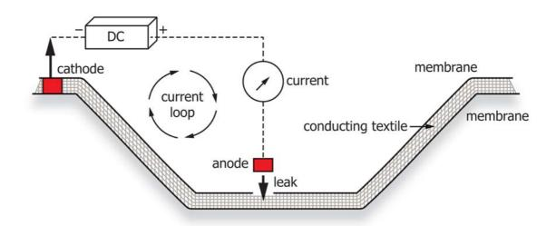
Schematic of leak detection with conducting geotextile
