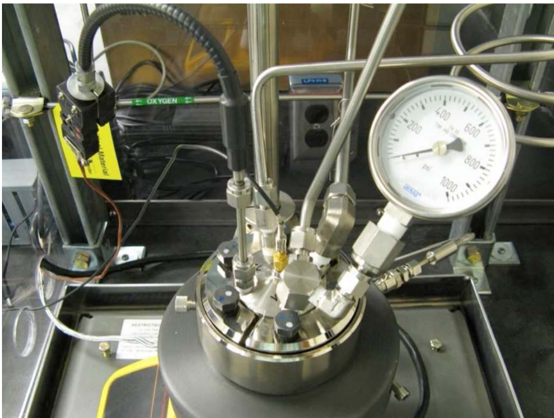
FIG. 5 Close-Up of Reactor (Skin Thermocouple Shown Below Dial Pressure Gauge)
