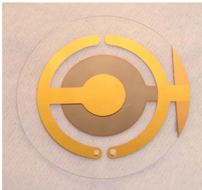
FIG. 2 Quartz Crystal (Front) Showing Proper Location of Indium Wire
