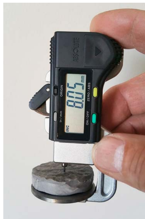
FIG. 2 Micrometer Measuring a Replica Coupon
