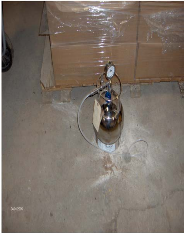
FIG. 4 Examples of Soil Gas Sampling Using Evacuated Canisters
