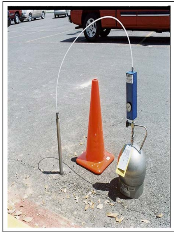
FIG. 4 Examples of Soil Gas Sampling Using Evacuated Canisters
