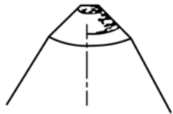
FIG. 3 Sketch of Abraded Shape of Extremity of Stylus After Testing Under a Microscope (5)
