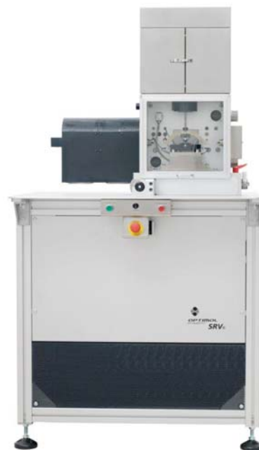
FIG. 3 SRV Test Machine (Model IV)
