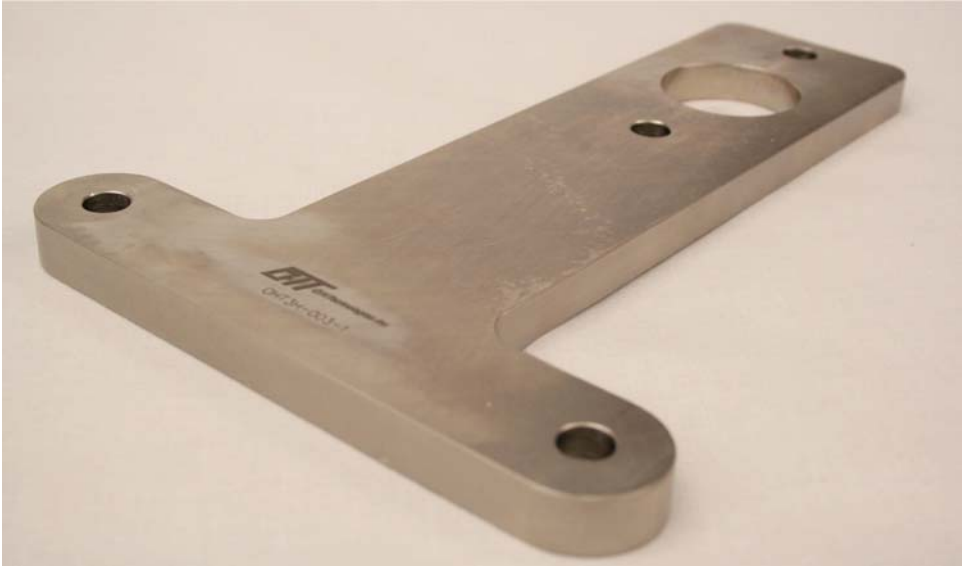
FIG. A5.19 Crankshaft Holding Tool
