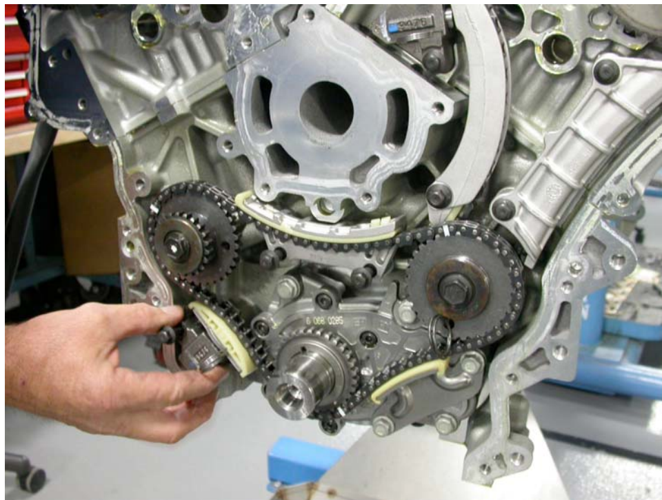
FIG. A17.9 View Showing Installation of Primary Chain Tensioner and Guides
