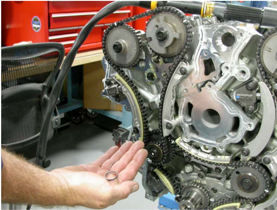
FIG. A17.13 View Showing Grenade Pins from Right Side Tensioner Removed
