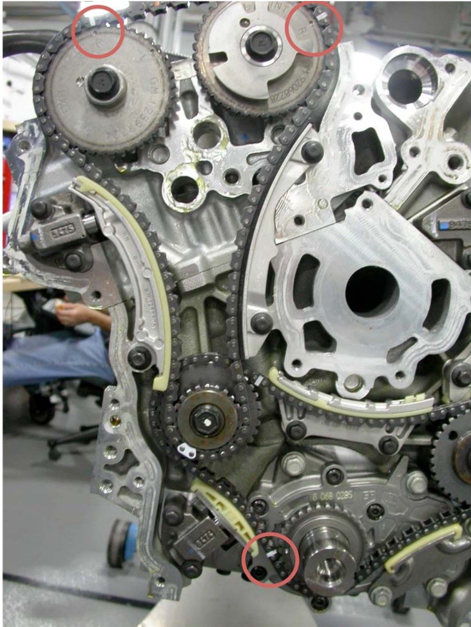
FIG. A17.15 Right Side Chain and Idler Alignment Marks
