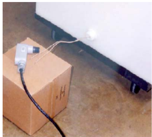
FIG. 7 TC Heater Installed in Tank Exterior
