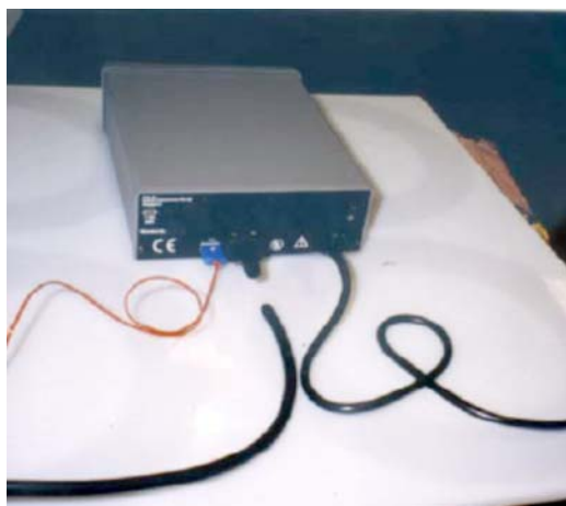
FIG. 9 Controller with connecting Cables: Power Heater Thermo-couple
