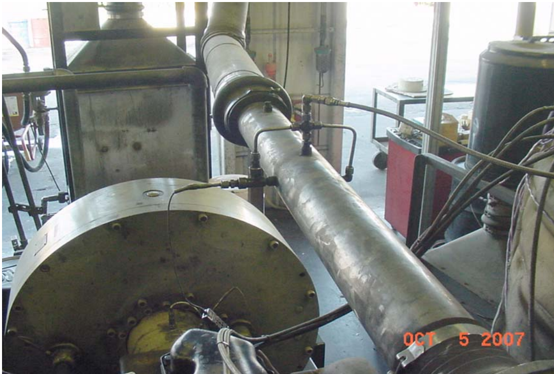
FIG. A4.2 Intake Air Temperature and Pressure Location
