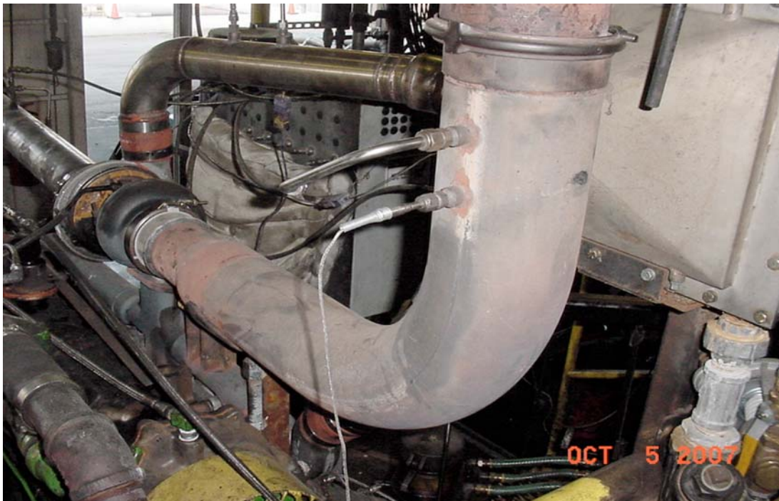
FIG. A4.7 Exhaust After Turbo Temperature and Pressure Location
