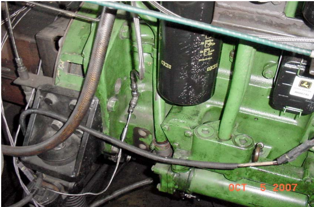
FIG. A4.8 Oil Gallery Temperature and Pressure Location
