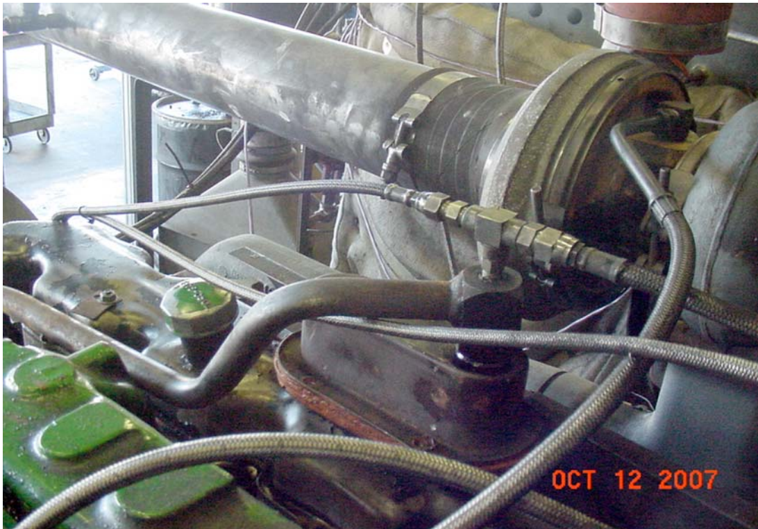
FIG. A4.10 Oil Fill, Blowby, and Crankcase Pressure Location
