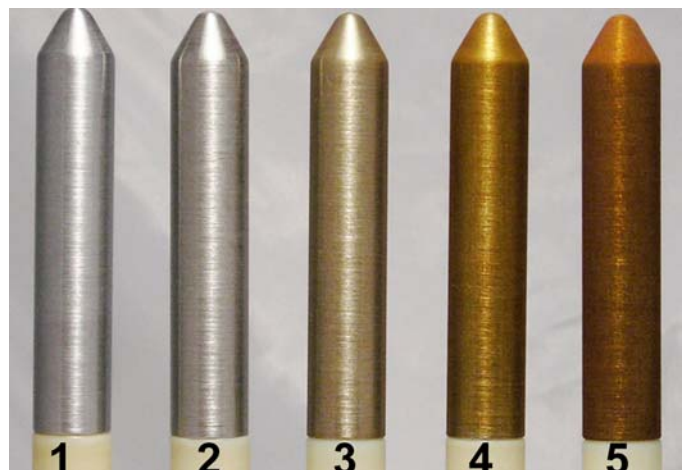
FIG. 3 Example of Visual Rating Scale. Photograph of Steel Test Rods at Each Corrosion Rating, Standards 1 to 5
