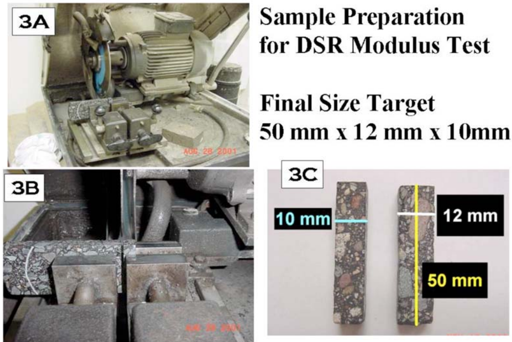
FIG. 3 Sample Preparation to Obtain 50-mm Wide by 12-mm Wide by 10-mm Thick Specimen.
