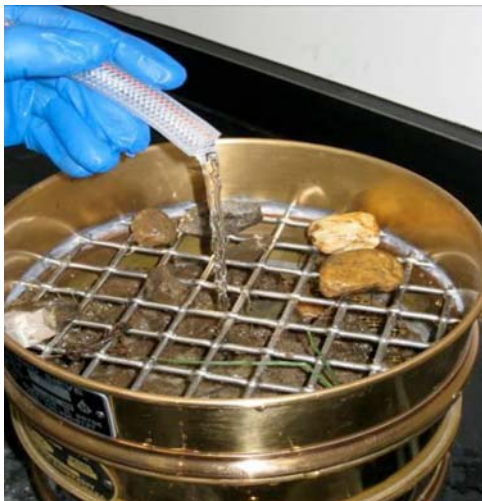
FIG. X1.3 Gently Wash the Course Fraction with a Gentle Stream of Particle-Free Deionized Water
