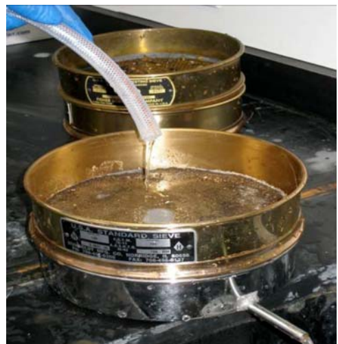
FIG. X1.5 Repeat Steps X1.8 and X1.9 for the >2-mm and >106- \mu m Fractions
