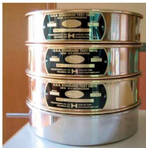
FIG. X1.1 Assemble a Sieve Stack from Top to Bottom as follows: ASTM 19-mm Sieve, ASTM 2-mm Sieve, ASTM 106-µm Sieve, and Collection Pan with Drain Outlet
