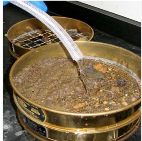
FIG. X1.4 Repeat Steps X1.8 and X1.9 for the >2-mm and >106- \mu m Fractions
