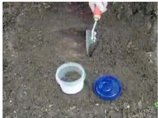
FIG. X2.2 Collection of Surface Sample: Loose Soil
