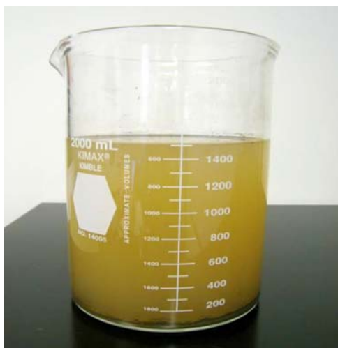
FIG. X1.6 Fine Fraction (<106 μm) that is in Suspension in the 2-L (or Larger) Straight-Walled Container is Covered and Set Aside for at Least 12 h to Allow the Particulate to Settle Out
