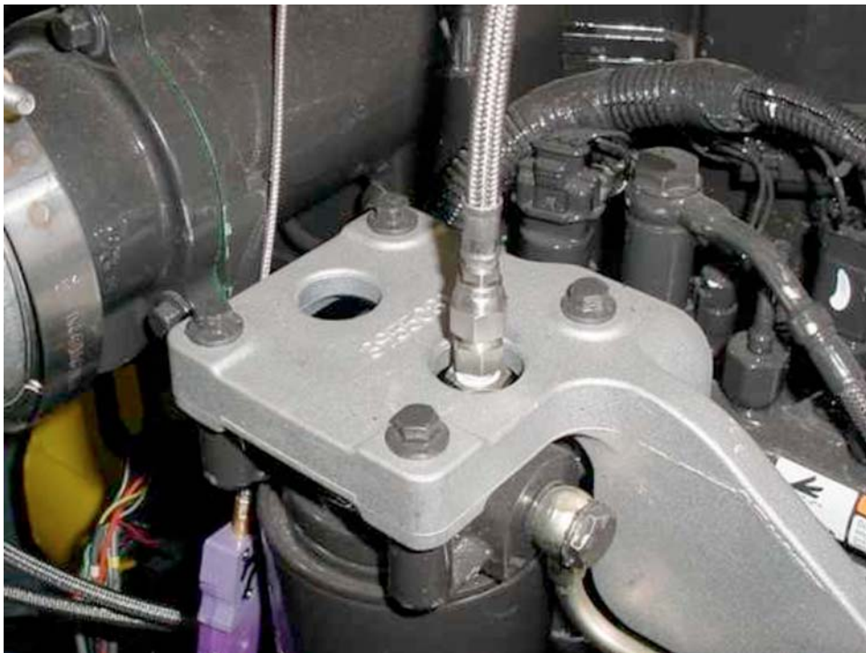
FIG. A4.14 Location of Sensor for Fuel-Pressure Measurement
