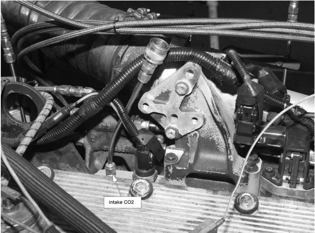
FIG. A4.14 Intake Manifold CO 2 Probe Location
