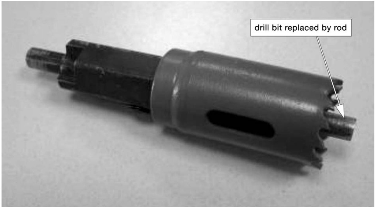
FIG. A4.16 Modified Hole Saw for Oil Capacitor Removal
