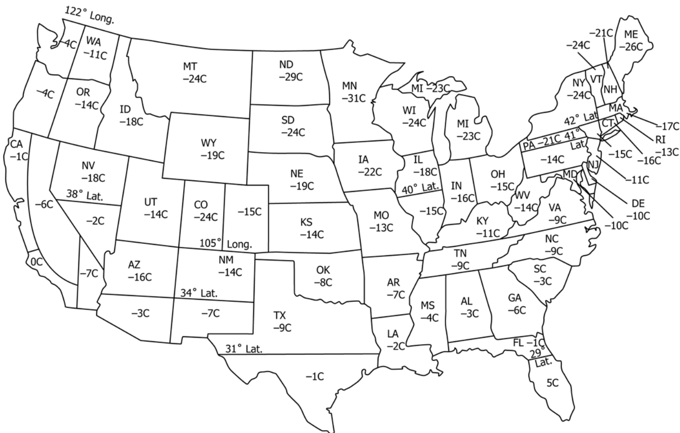
FIG. X3.5 February—10th Percentile Minimum Ambient Air Temperatures
