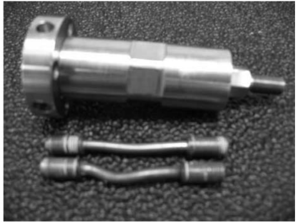
FIG. 5 Tensile Bar Coupler Connecting the Actuator to the H-frame (Inner Clamps)
