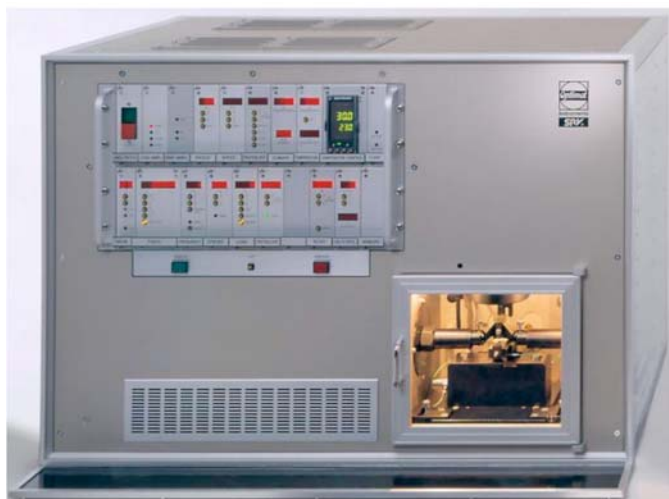
FIG. 1 SRV Test Machine (Model III)
