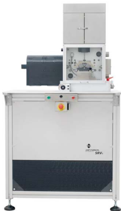
FIG. 3 SRV Test Machine (Model IV)
