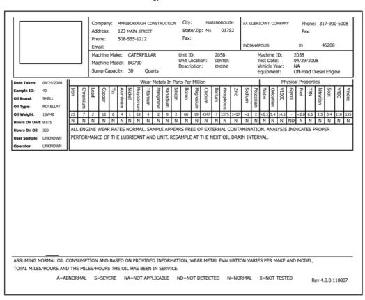
FIG. X1.1 Example of Extended Metals and Wear Report
