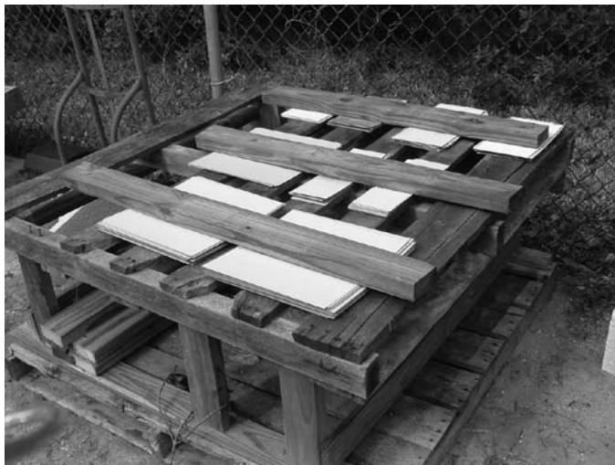
FIG. 1 Illustration of Wet Stack Test Placed Horizontally (Level) on a Pallet
