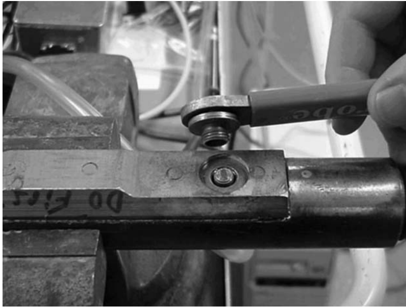
FIG. A1.1 Membrane Wrench Shown with Membrane Removed Exposing the Sub-Membrane Fittings
