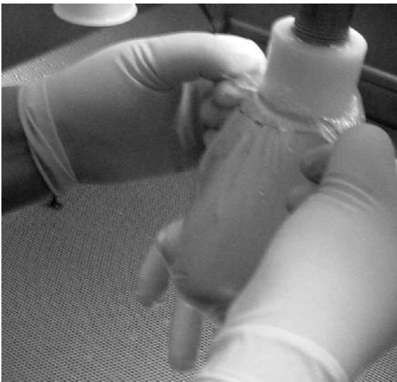
FIG. 5 Removing Test Sample from Mandrel
