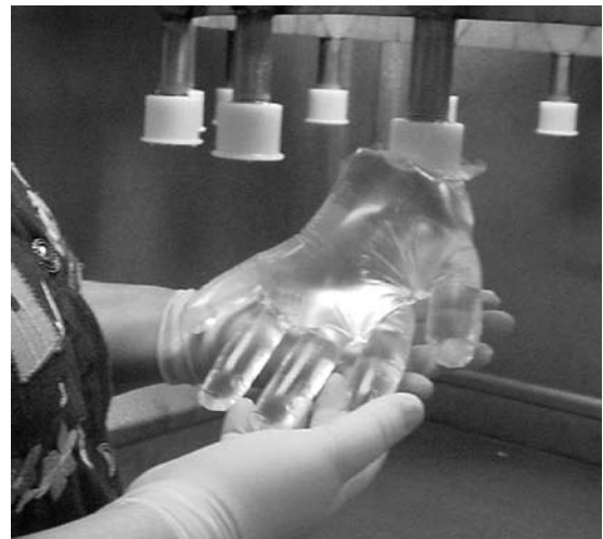
FIG. 3 Lifting Test Sample to Examine for Defects
