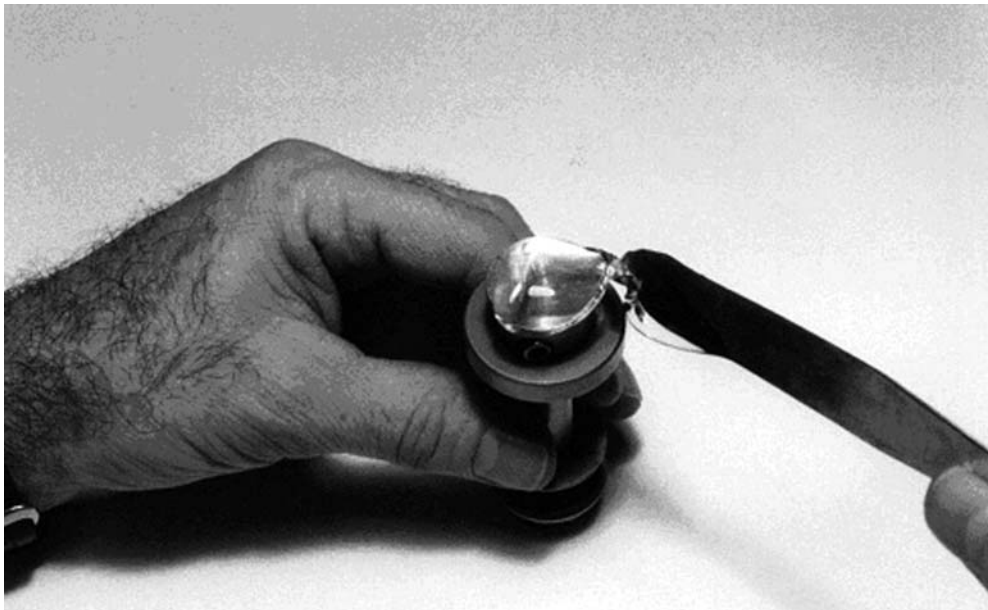
FIG. A1.2 Using a Spatula to Place the Reference Fluid on the Plate
