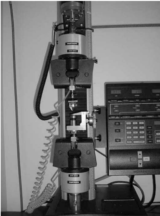
FIG. 2 CRE-Type Tensile Testing Machine setup With Test Fixtures For Option 1.
