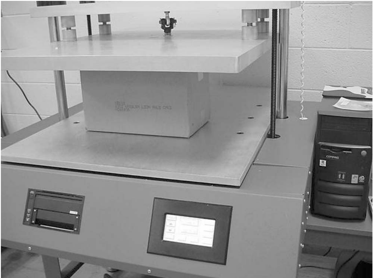
FIG. 1 Corrugated Container Under Creep Test in Compression Test Machine
