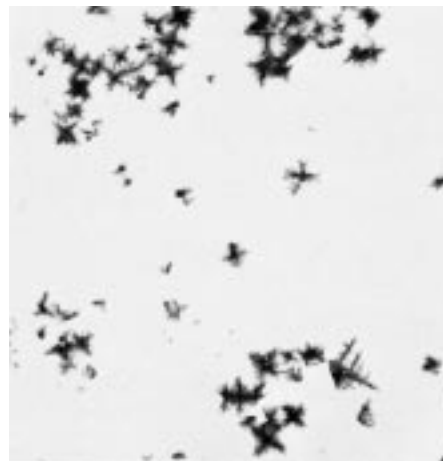
FIG. 12 Zinc Mercuric Thiocyanate Crystals ( \times 75 )
