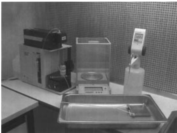
FIG. 1 Illustration of Apparatus to Determine Dynamic Wiping Efficiency, Wet Particle Removal Ability, and Fabric Particle Contribution
