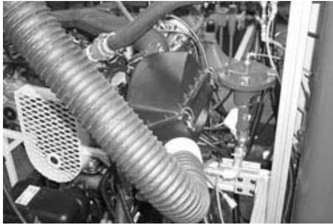
FIG. A7.21 Intake Air Supply System, Air Cleaner, Resonator and Idle Load Control
