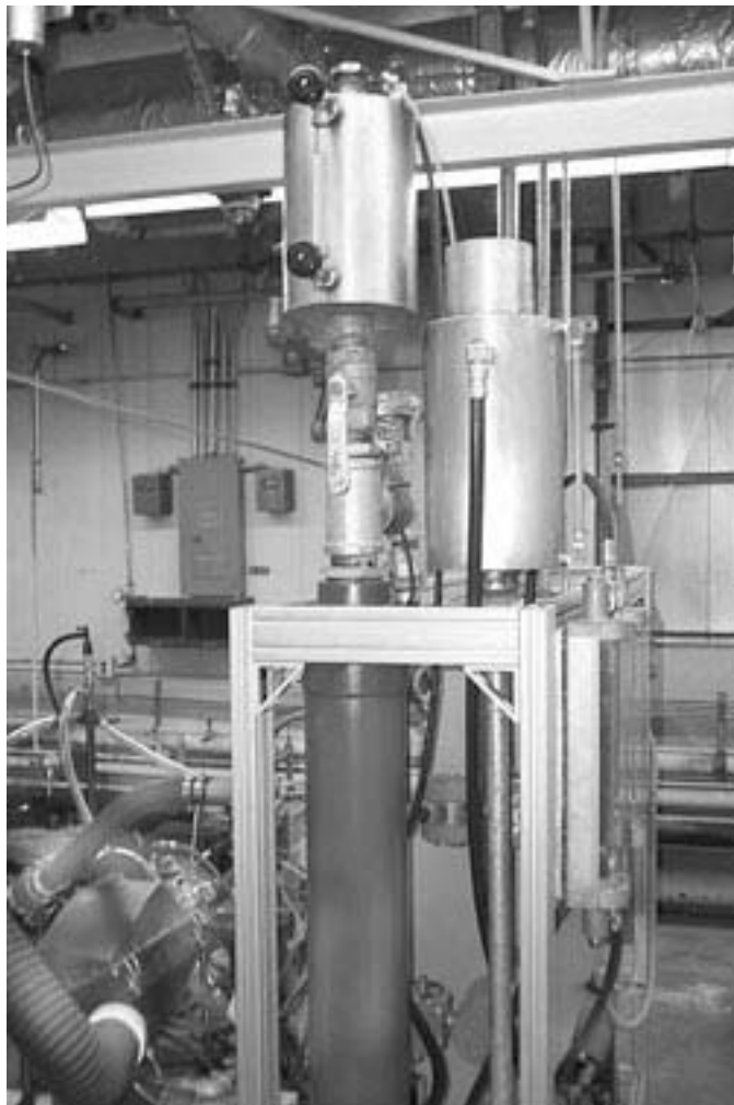
FIG. A7.22 Typical Engine Cooling System, Venturi Flowmeter
