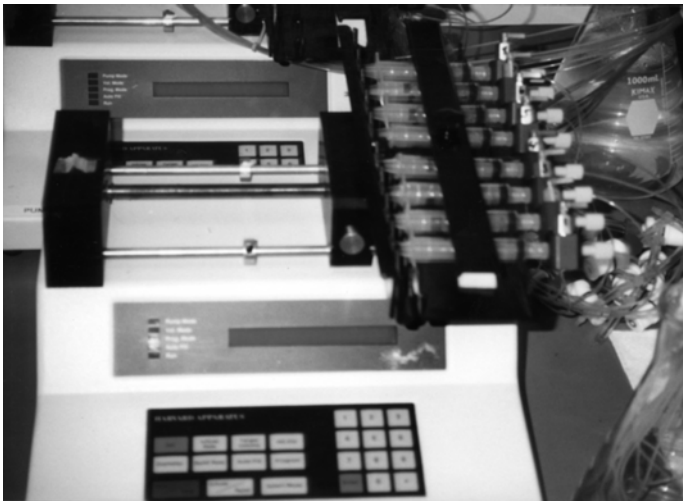
FIG. 3 Photograph of Acid Delivery System
