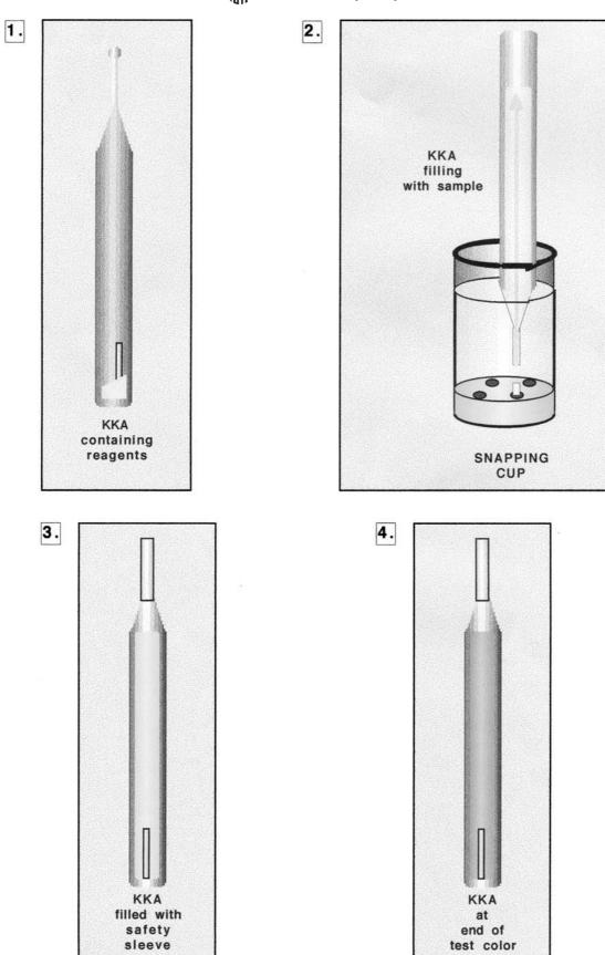
FIG. 1 Schematic of Kool Kount Test Kit
