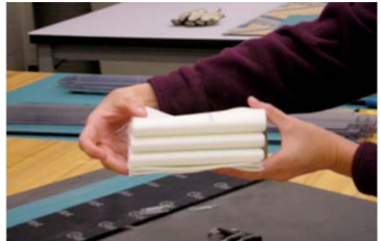
FIG. X1.15 Example of Folded Specimen
