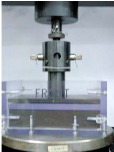
FIG. X1.4 Specimen Box with 30 mm Block
