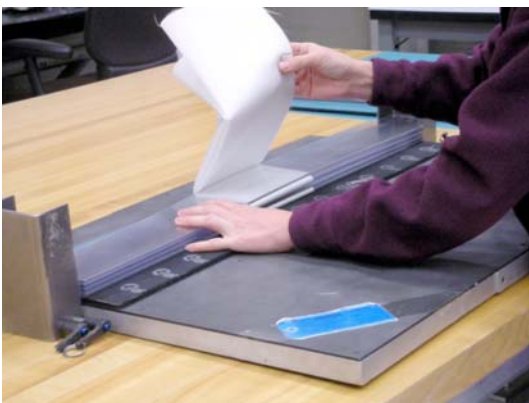
FIG. X1.13 Folding Specimen Using Narrow Slats
