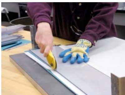
FIG. X1.7 Trim Excess Fabric Using Rotary Cutter
