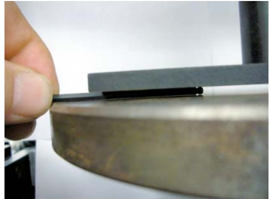
FIG. X1.2 Checking for Parallel Alignment
