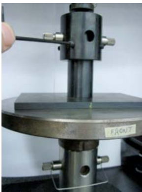
FIG. X1.1 Locking Compression Foot
