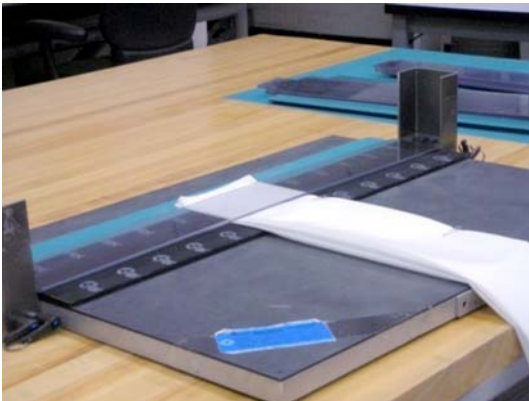
FIG. X1.12 Position Folded Stack and Align Edges
