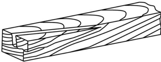
SPIRAL AND DIAGONAL GRAIN IN COMBINATION
