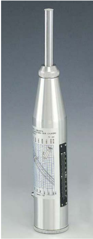
FIG. 1 Typical Rebound Hammer with Correction Graph for Non-Vertical Use and Rebound Scale on the Side of the Body for Manual Readings
