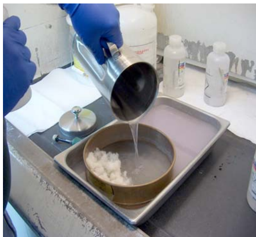
FIG. 8 Cleaning the Blender Out by Pouring Residue Into Clear Area of the Sieve
