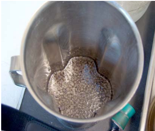
FIG. 3 Buried Yarn with Chloroform, Before Mechanical/Blender Separation
