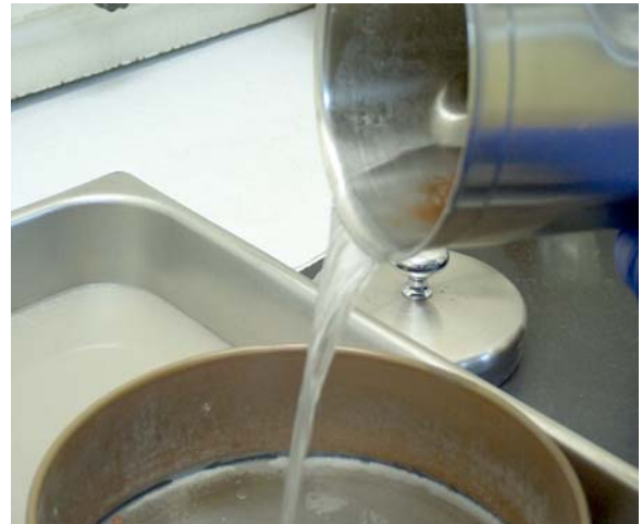
FIG. 6 Separation of Latex from Fiber with Solvent (Note Clear Solvent Color Indicates No Latex is Present in the Specimen)
