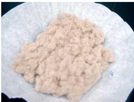
FIG. 9 Buried Fiber After Separation from Latex Compound, Placed on Pre-Weighed Paper
