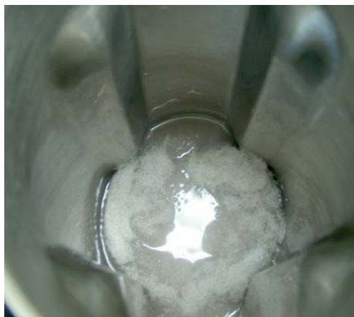
FIG. 4 Yarn Separated from the Latex Compound
