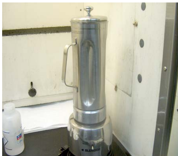
FIG. 1 Two Quart Blender Typically Used to Mechanically Separate Buried Yarn from the Latex Compound
