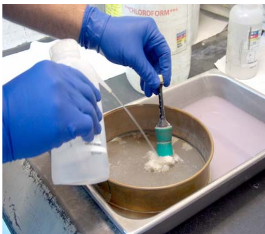
FIG. 7 Using Presser Tool and Chloroform to Break Up Hard Pieces of Buried Fiber
