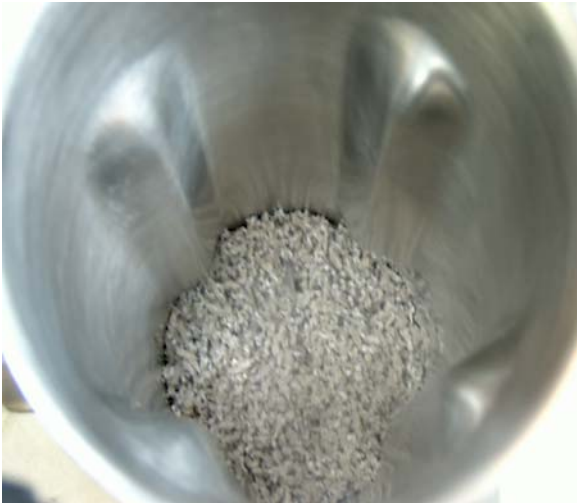
FIG. 2 Buried Yarn in Blender (Before Chloroform Addition)
