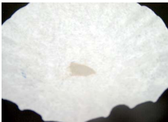
FIG. 10 Residual Compound Held in Sieve and Placed on Pre-Weighed Paper
