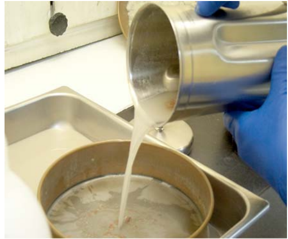
FIG. 5 Separation of Solvent from Fiber (Note Milky Solvent Color Indicates Latex is Still Present in the Specimen)
