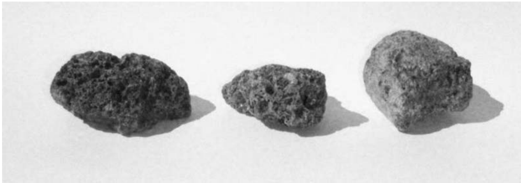
FIG. 4 b) Fractured Particle (Round Edges, Rough Surfaces) (continued)
