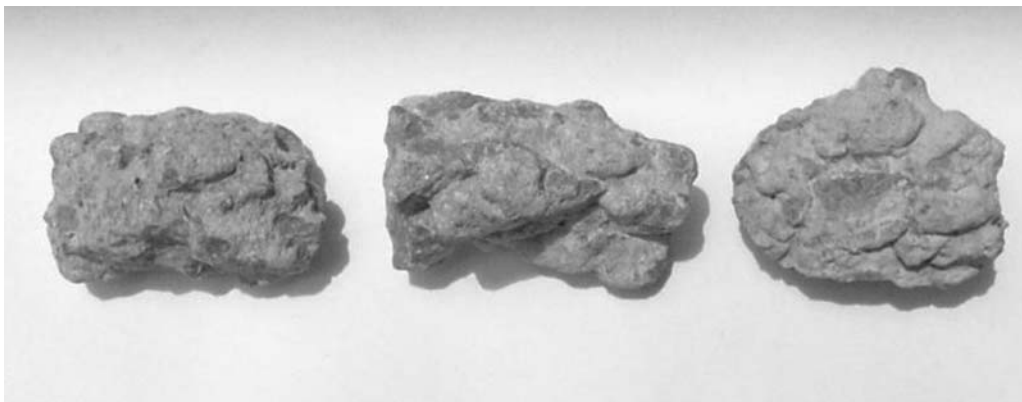
FIG. 4 c) Fractured Particle (Round Edges, Rough Surfaces) (continued)
