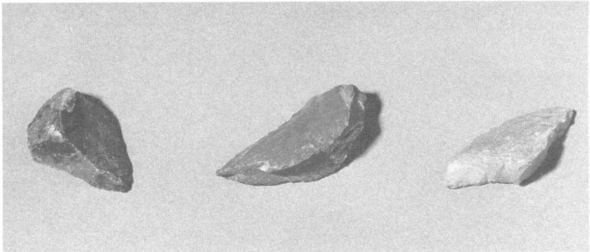
FIG. 3 Fractured Particle (Sharp Edges, Smooth Surfaces)
