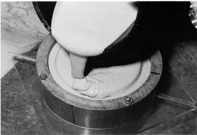
FIG. 3 View Showing Pouring Encapsulating Material Around Upper Half of Specimen
