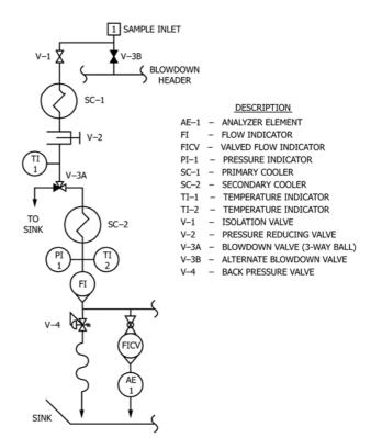
Note 1—Fixed back pressure regulating valves (V4) are available and eliminate the need to adjust back pressure and readjust the flow. This fixed pressure regulating valve provides the added benefits of acting as a sample relief valve and grab sample discharge.
