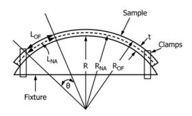
R = radius of jig  $R_{NA} = radius of neutral axis$  $R_{OF} = radius of outer fiber$
