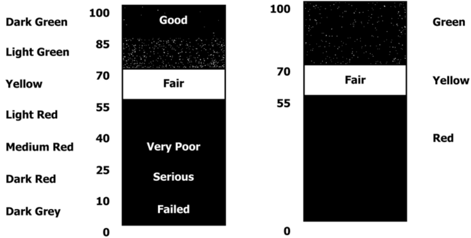
FIG. 1 Two Examples of Pavement Condition Index (PCI (trademarked)) Rating Scales
