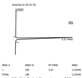
FIG. X2.3 Typical Chromatogram—DPG
