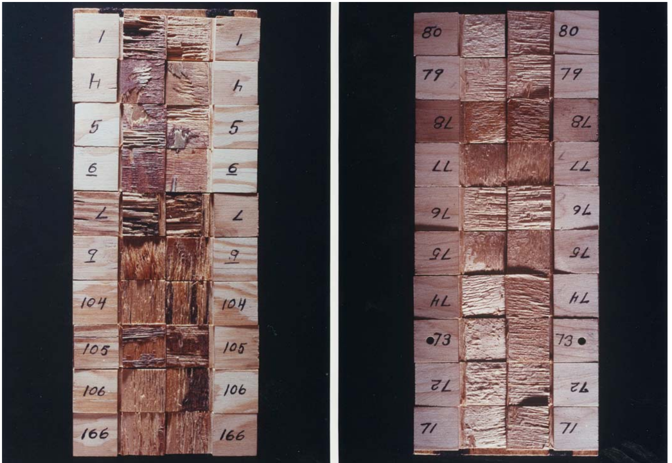
FIG. X1.1 Visually Estimating the Percentage of Wood Failure in Standard Adhesively Bonded Specimens (Left) Three-ply, Douglas-fir, Phenol-formaldehyde adhesive. (Right) Three-ply, Yellow-birch, Urea-formaldehyde adhesive.
