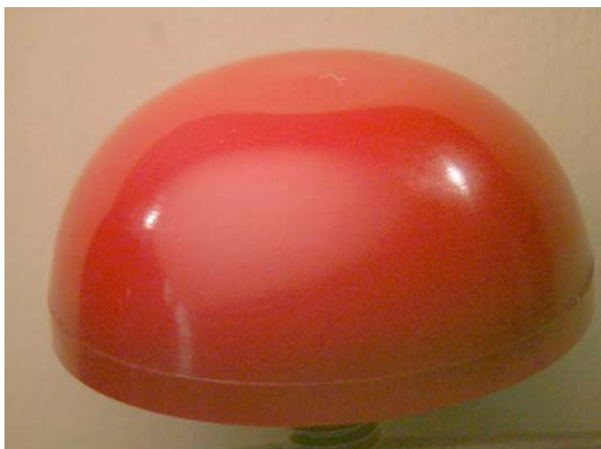
FIG. 5 Typical Hexapod Tumbler Foot
