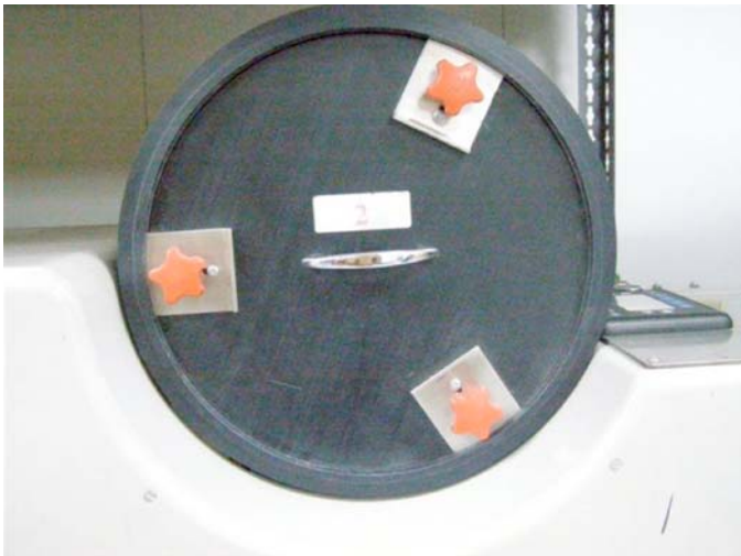
FIG. 1 Typical Front View of Drum Cover
