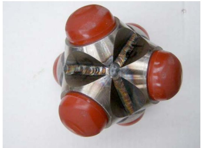
FIG. 3 8.4 lb Commercial Hexapod Tumbler
