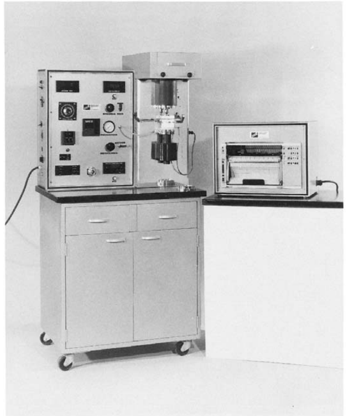
FIG. 2 Falex Variable—Speed Four-Ball Wear Test Machine
